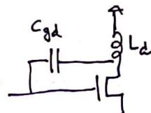
$$\rightarrow C_{gd} \text{ transfers } L_d \text{ to negative } R. \quad Y_{in} \text{ from } C_{gd} \approx C_{gd}(1+A) \approx jwC(1+g_m jwL) \\ \approx -w^2 g_m C_{gd} L_d$$
